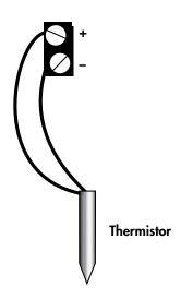
Wiring a Temperature Sensor
