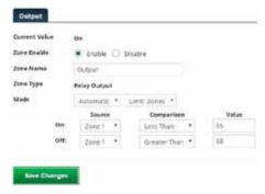
Action - This setting determines what the Output will do when the selected zone (or zones) exceeds the alarm limits. You can have the relay Activate (turn-on), Deactivate (turn-off), or Cycle (ON under normal conditions, momentarily OFF for 10 seconds when an alarm condition occurs, then back ON).
