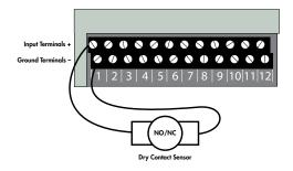
Wiring a Dry Contact Sensor
