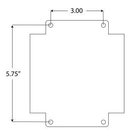
Figure 2: Sentinel Pro mounting dimensions
